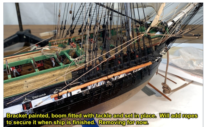
Since I was turning the yards, I also turned the two stunsail booms for the foremast. Needed brackets to support the ends, so I bent some brass, soldered them together, and mounted near the end of the boom.
