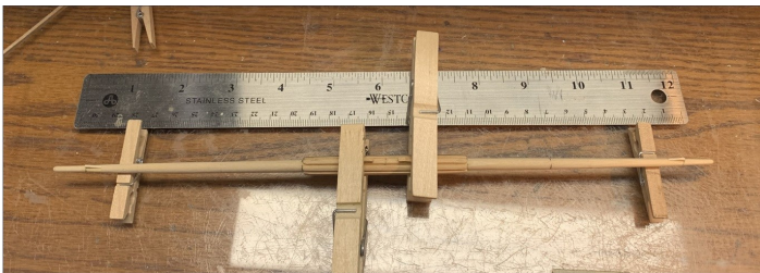
Turning of mainyard complete; adding all the battens and dogs.
